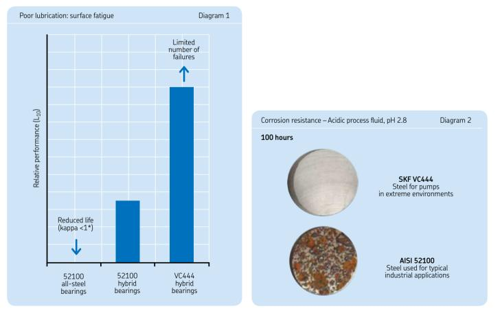
Under poor lubrication conditions, SKF super-tough VC444 stainless steel resists surface fatigue nearly three times as long as standard hybrid steel.(Diagram shows SKF in-house life test results.)
